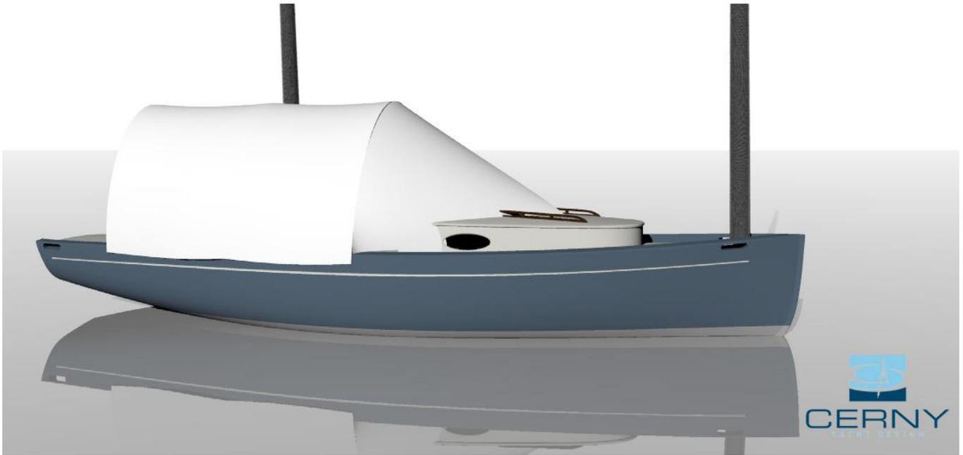
The cabin can be extended out into the cockpit with a quick and easily assembled cockpit tent. The sprit booms are quickly disconnected from the masts to make room for this standing headroom living space.
